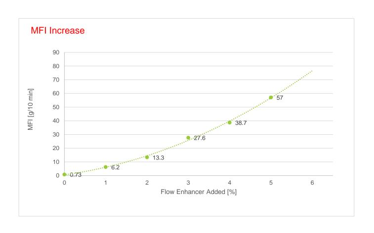
GRAFTALEN™ SA is an additive for polymers, used for regulating rheological properties and as release agent for injection molding.
